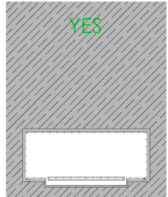
**DO!** install the fireplace in a massive wall (made of bricks, stone or gas beton) using the wall cut-out dimensions mentioned on the previous page.
