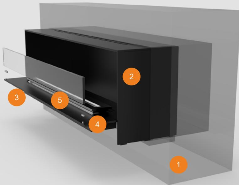
**Step 1:** Make sure that the dimensions of the cut-out correspond to the measurements indicated in the technical drawing received with your fireplace. Also be sure there is no draft inside the wall.
